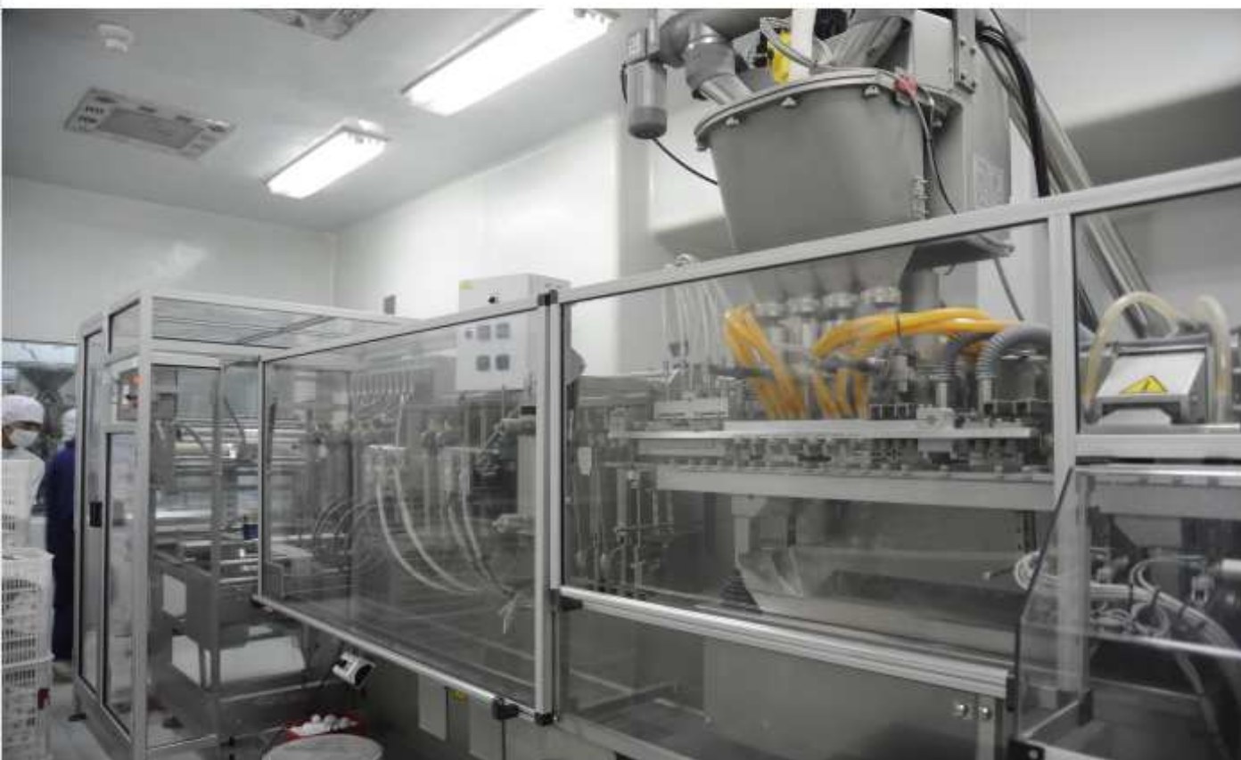
Four-sachets filling machines in Factory 5
